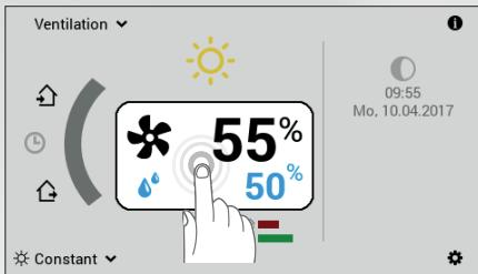
Adjust the air quantity and max. air humidity using (+/-) or by entering directly (tap the value) and confirm with OK.
