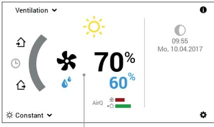
The air quantity and limit value for max. air humidity rise/fall to the required value.
