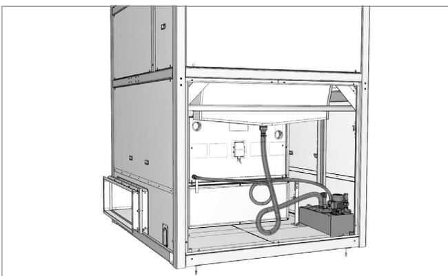
Fig. D11: Return pump station installed in the unit
