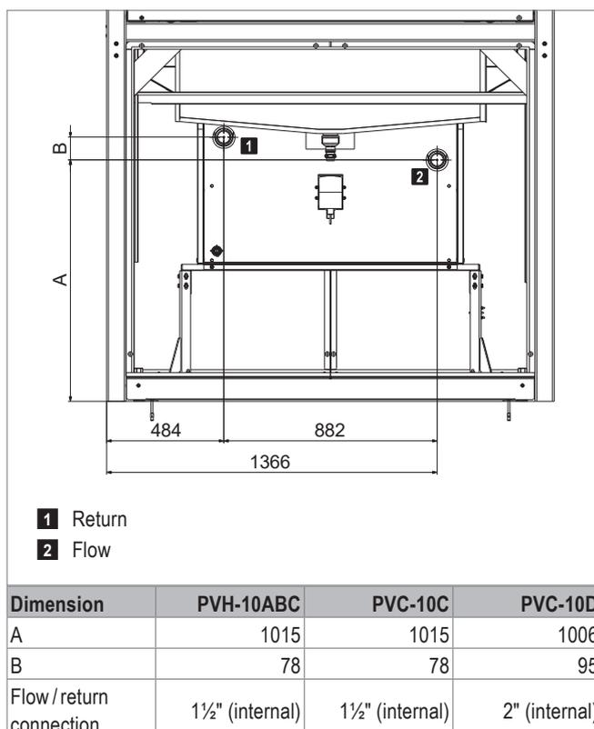
Fig. E5: Dimensional drawing for hydraulic connections (dimensions in mm)
