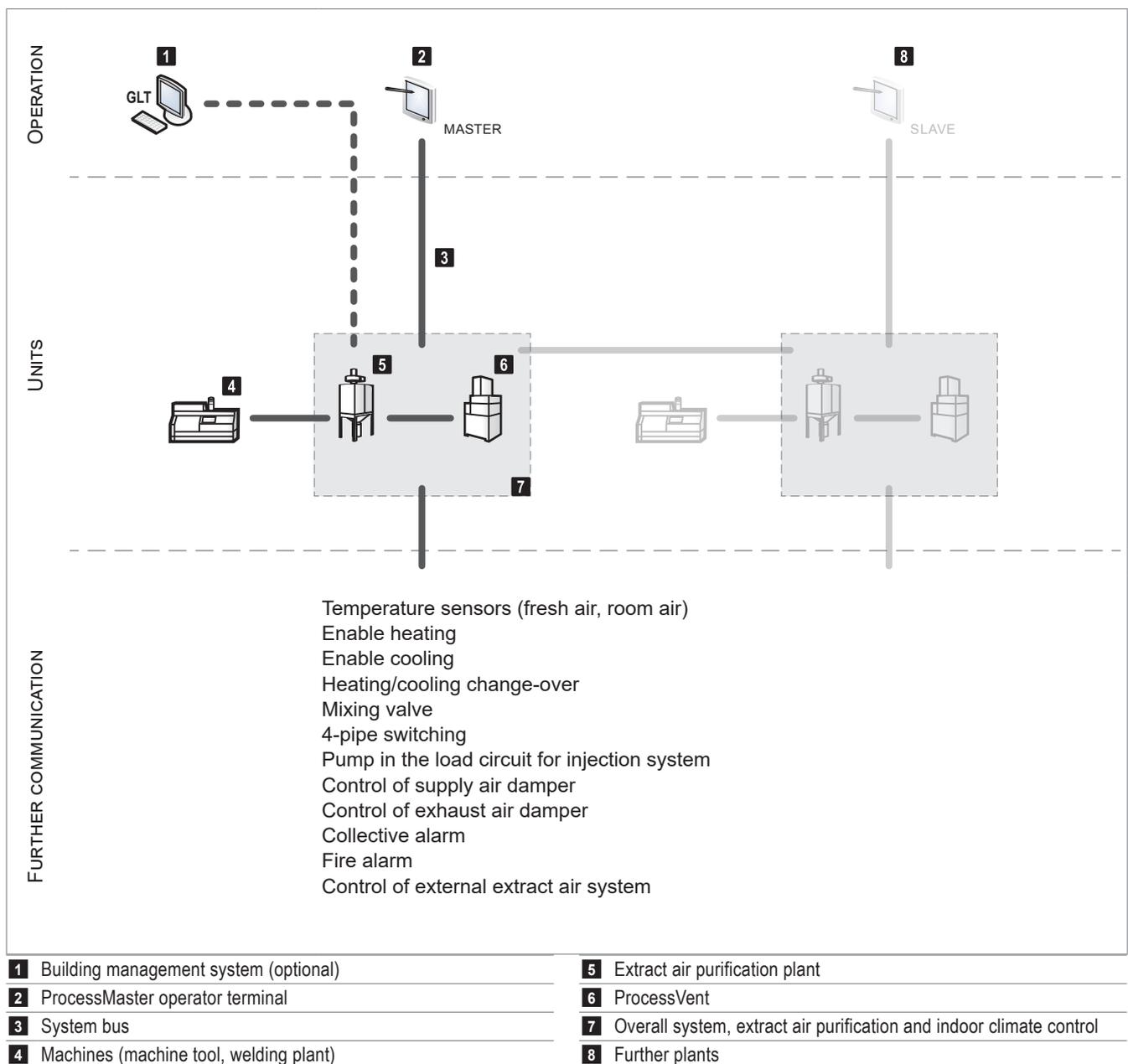
Fig. G1: ProcessNet system set-up
