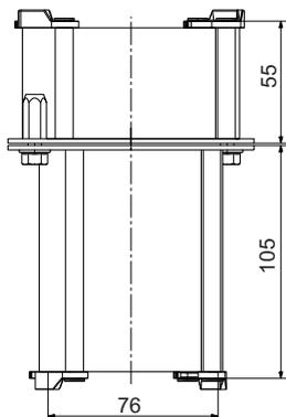
**Formwork coupling SK-75/90**
