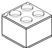
**Acoustic insulating box FRT extract-supply air front**
