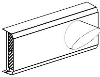
**Wall outlet Ø 160 exhaust air on right**
