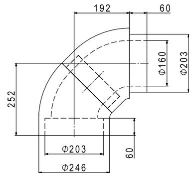
**IsiPipe Plus pipe system EPP-200**
