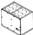
**Acoustic insulating box for plywood 12 x 90**
