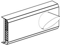
**Wall outlet white Ø 160 exhaust air on right**
