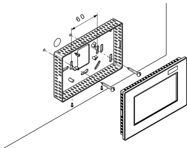
**Wall mounting with wall mounting plate**
