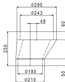
IsiPipe Plus device adapter EPP-200
